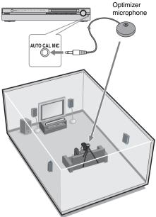
1 Connect the supplied optimizer microphone to the AUTO CAL MIC jack.
